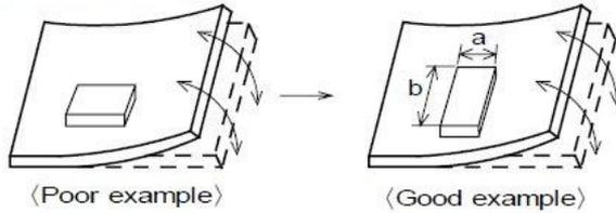
Products shall be located in the sideways direction (Length: $a < b$ ) to against the mechanical stress.
