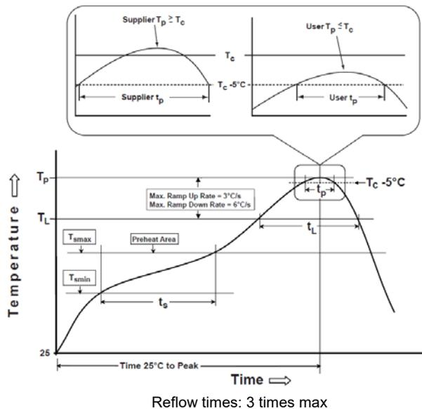
Fig.2 Iron soldering temperature profiles
