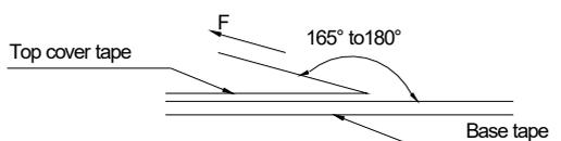
The force for tearing off cover tape is 10 to 80 grams in the arrow direction under the following conditions (referenced ANSI/EIA-481-C-2003 of 4.11 standard).
